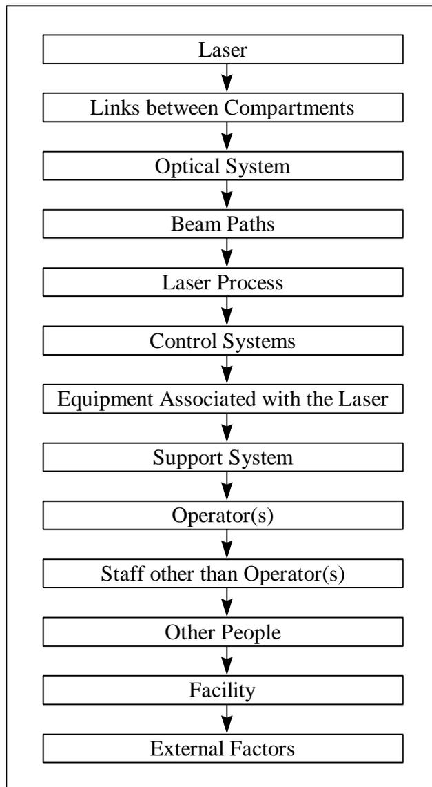
Figure 8.3 Industrial Laser Hazard Methodology
