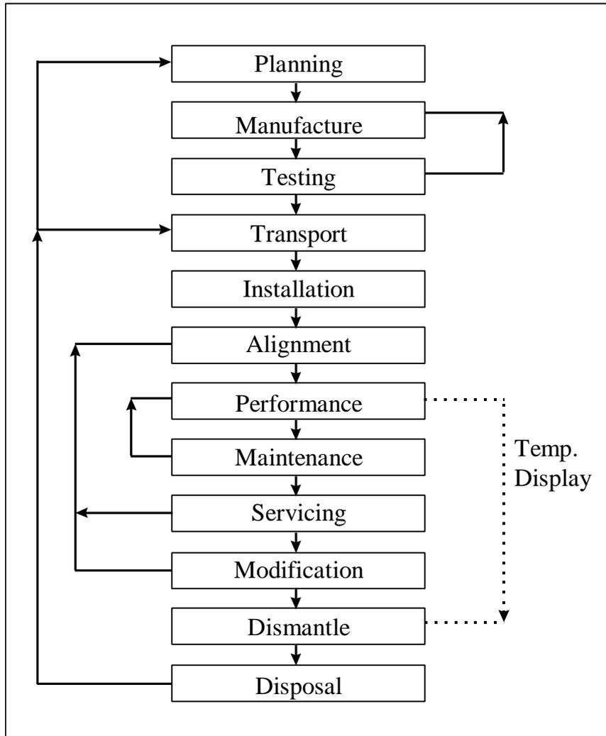
Figure 6.1 Life Cycle of a Typical Laser Display
