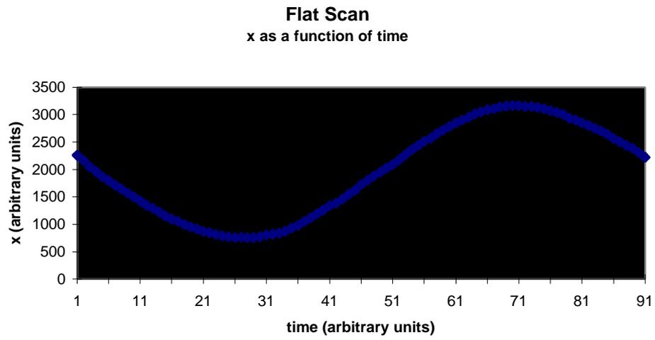
Figure A.1 Values of x as a function of time for a flat scan (y is constant)
